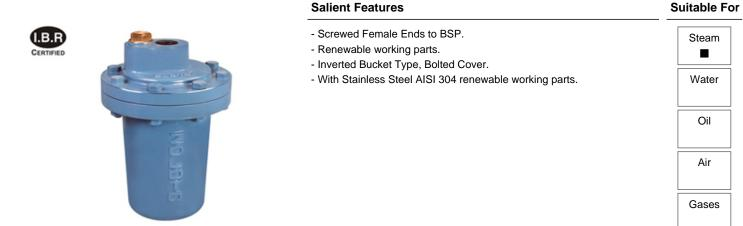
Test Pressure (Hydraulic) Shell : 21.10 kg/cm<sup>2</sup>g (300 psig) Maximum Working Pressure : 10.55 kg/cm<sup>2</sup>g (150 psig) Maximum Working Temperature 220°C
