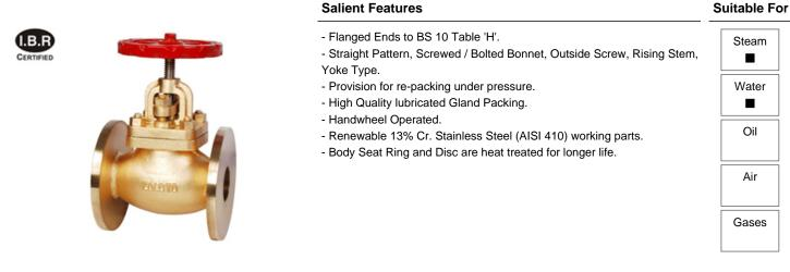
Test Pressure (Hydraulic) 35.15 kg/cm<sup>2</sup>g (500 psig) Working Pressure (Steam) 17.58 kg/cm<sup>2</sup>g (250 psig) Maximum Working Temperature 225°C
